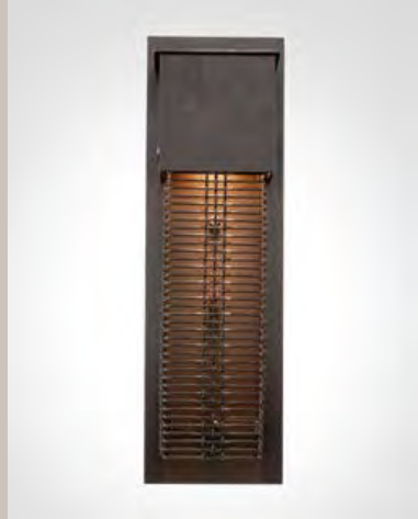
Short Square Mesh Cover Sconce ODB0040-16-SB-M2 OAH 16.2" W 5" D 3.7" GU10 Base ADA Compliant Wet Rated
