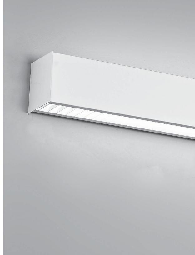
Housing: Fabricated from die-formed, 20-gauge, cold-rolled steel. Ballast compartments provided with 7/8"-diameter KOs at either end of housing for through wiring.
