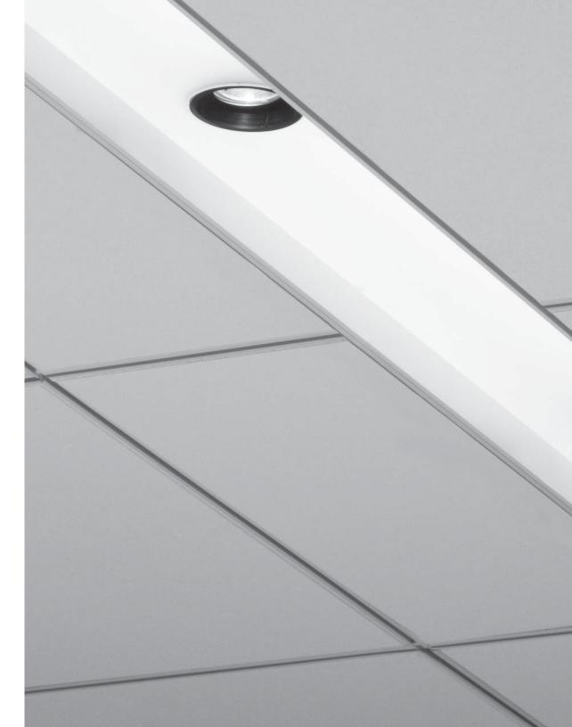
Housing: Nominal 6" wide x 2', 3', 4', 5', 6' or 8' long housing fabricated from 20-gauge, cold-rolled steel. Ceiling trim is extruded aluminum. Downlight component is die-cast aluminum.
