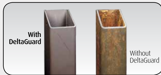
The same 3-mil thickness of powder was applied to each of these two pole section samples. Each was scored and exposed to a salt-fog test for 2,500 hours.
